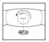
Remove the old battery from the sensor unit. Insert a new CR 2032 battery, making sure that the writing is on top. In addition, make sure that the rubber gasket is in place in the sensor unit. Replace the battery cover and turn it to the closed position.
